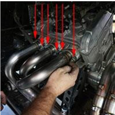
19. Align the header collector with the mid-pipe flange and install the v-band clamp.
