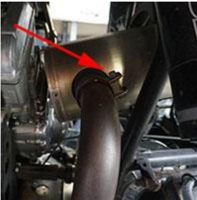
3. Remove the header. It will be easier if you remove the front first then wiggle the rear out of the muffler.
