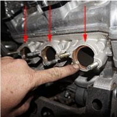
18. Install the header. Start the 6 nuts and snug by hand. Tighten @ step 20.
