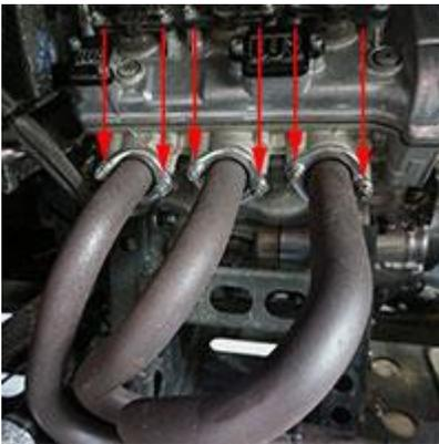
4. Remove the 4 bolts holding the muffler on using a 14mm socket.
