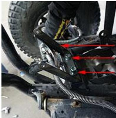
**12. Install the new mufflers using the M8 bolts, nuts, and washers. Leave snug until step 20.**
