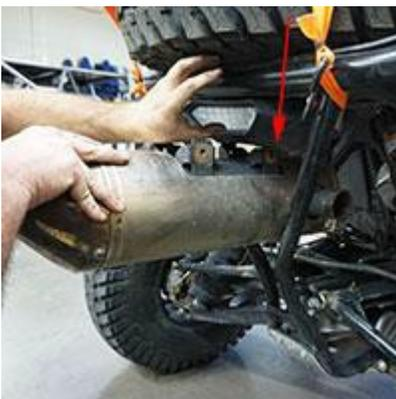
**10. Rotate the muffler one last time to clear the rear frame rails and pull out.**
