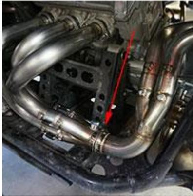
20. Now tighten the v-band clamp and all the mounting bolts. Also, re-install the 2 springs removed earlier from the rear mid-pipe.
