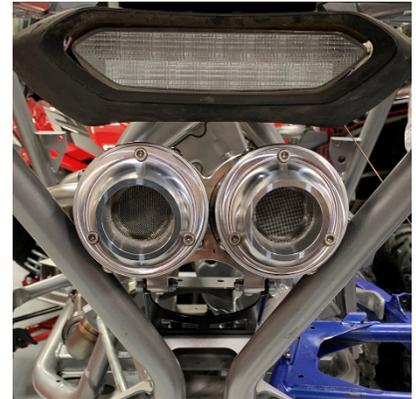
**14. Remove the springs and 2 pipes from the merge collector.**
