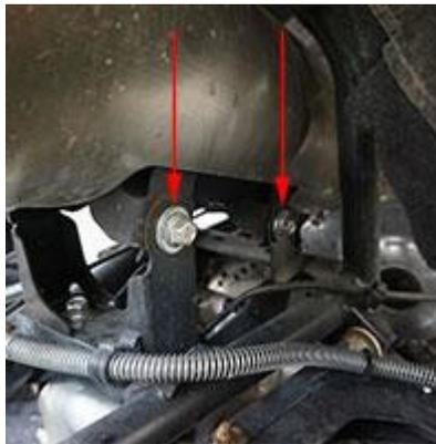
6. Remove rear lower bracket bolts and bracket using a 14mm socket.
