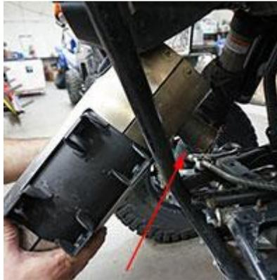
**11. Install the supplied lower bracket as shown. Red Loctite the bolts and leave snug until step 20.**
