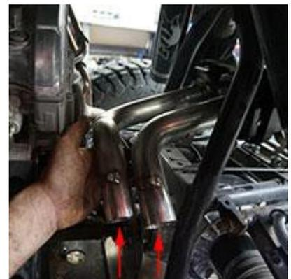
16. Re-connect the merge connector. Re-install the springs at step 20.
