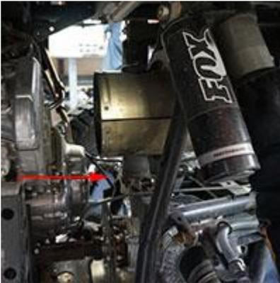
**8. Once you get to this point, rotate the muffler as shown and keep fishing it out.**
