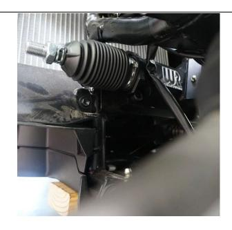
30. ADJUST THE TOE SETTING BY COMPARING THE FRONT AND THE REAR OF THE TIRE AT THE SAME HEIGHT. THE FRONT SHOULD BE 1/8" TO 1/4" WIDER THAN THE REAR FOR A TOE OUT SETTING LIKE WE RUN. WHEN YOU ARE DONE, BOTH SIDES SHOULD BE SIMILAR IF EVERYTHING IS CENTERED PROPERLY. IF NOT, THEN YOU WILL NEED TO REMOVE YOUR STEERING WHEEL AND ADJUST IT TO ONE SIDE OR THE OTHER TO CENTER IT TO THE RACK.
