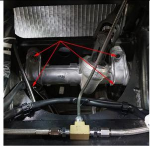
**7.** REMOVE 4x RACK MOUNTING BOLTS USING A 12mm SOCKET (SAVE FOR RE-USE)
