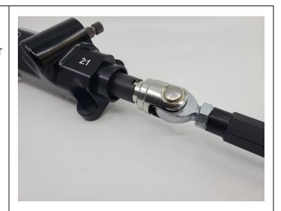
17. CENTER THE STEERING RACK BAR. USING CALIPERS OR TAPE MEASURE, MEASURE HOW FAR THE RACK BAR IS STICKING OUT OF THE HOUSING. CENTER IS 0.97"(1") OUT THE DRIVER SIDE AND 1.27"(1-1/4") ON THE PASSENGER SIDE. MARK THE TOP OF THE RACK HOUSINGS TO SPLINES WITH PAINT MARKER TO KEEP CENTERED AFTER BOOTS ARE INSTALLED.
